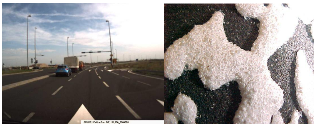
Figure 3 - Start position on tested field and structure of road markings (state road D31)
