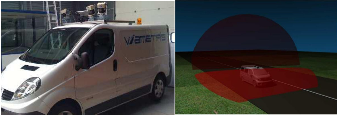
Figure 1 - Shows vehicle equipped with lidar and cameras while figure 2 shows “Front” and “Sky” lidar sensors cones of view
