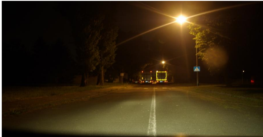
Figure 3 - Show different visibility of two vehicle – one vehicle is with contour marking and the other is without contour marking
