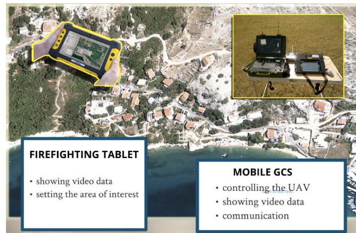
Figure 5 - Mobile systems for communicating and/or receiving on-board sensors data [7]
