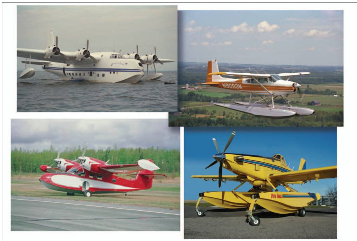
Figure 1 - Seaplane (a seaplane landing on the hull, a seaplane with floats, amphibian – capable of landing on both land and water)
