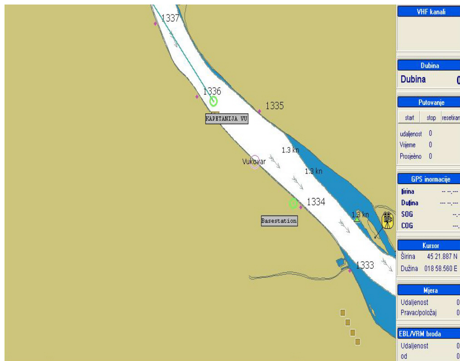
Figure 2 - Sample of Electronic Navigation Chart in accordance with the Inland ECDIS standard installed on a computer
