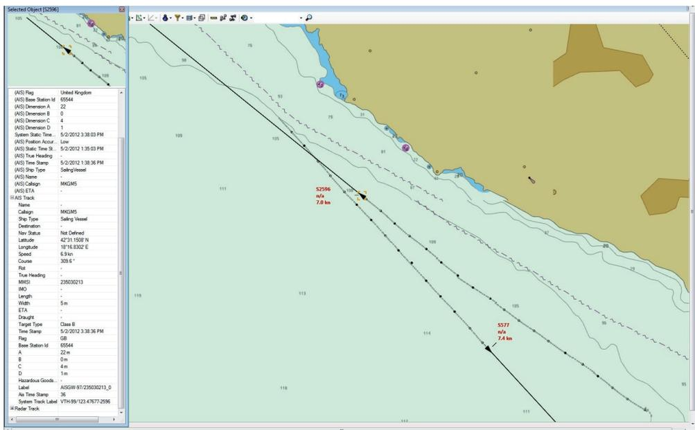
**Figure 3** Presentation of AIS Class B on the VTS operator's control display (SAAB CoastWatch VTS Software)
