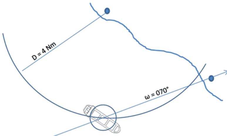
**Figure 2** Position fix with a bearing on and the distance to two conspicuous objects
