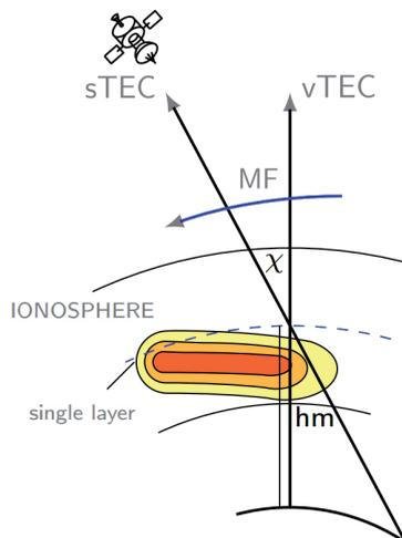
**Figure 2** Thin shell approximation of the ionosphere
