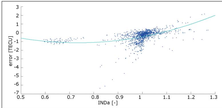
**Figure 7** Statistical regression of TEC error to asymmetry index
