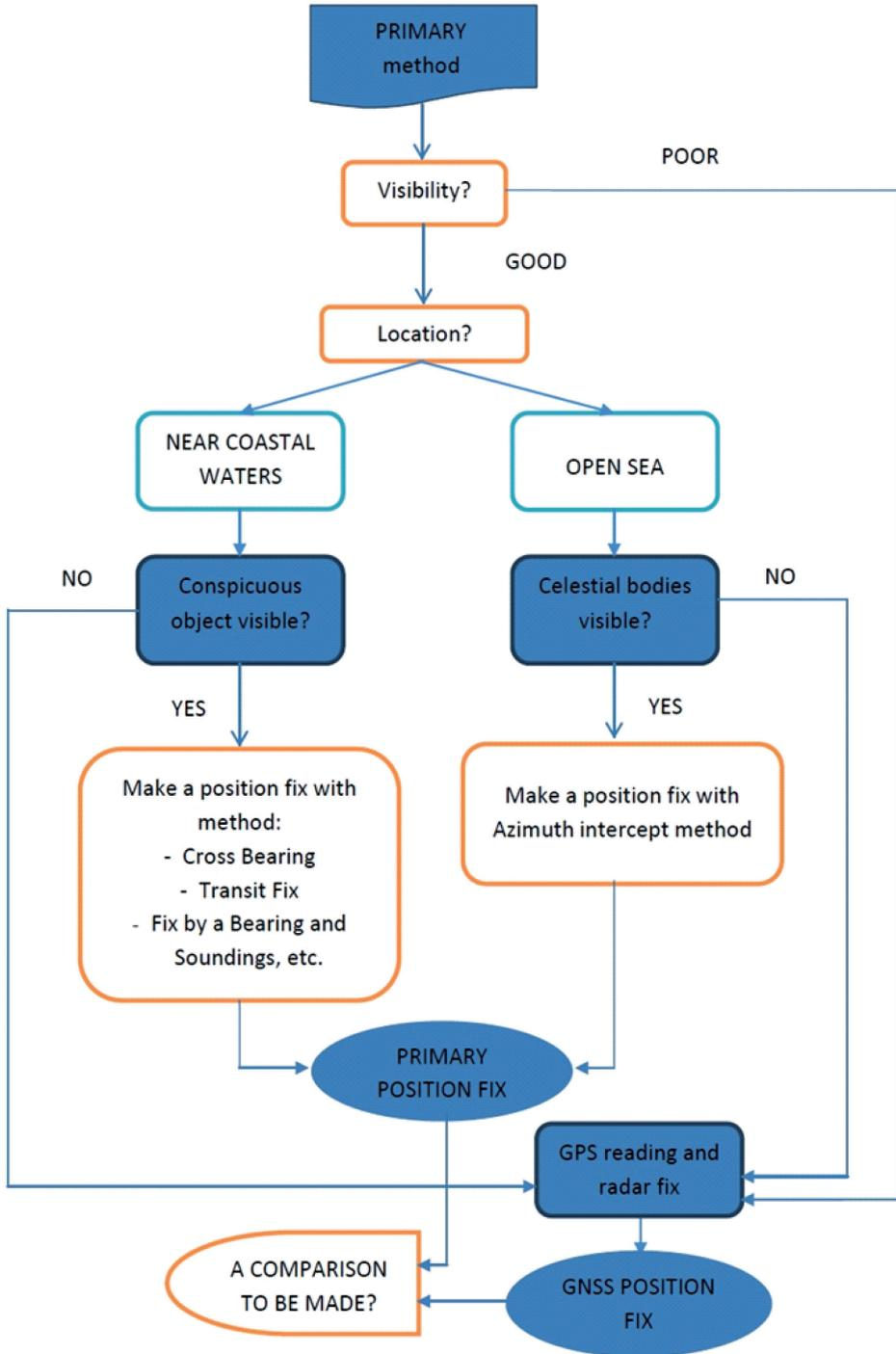
Figure 3 The position getting algorithm – the safe way
