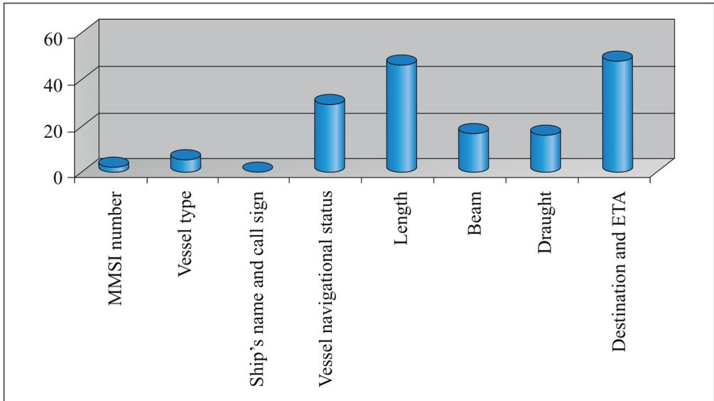
**Figure 5** The most common AIS message errors, given in percentage
