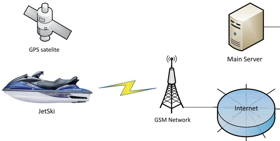
**Figure 7** Block diagram of the proposed tracking system architecture
