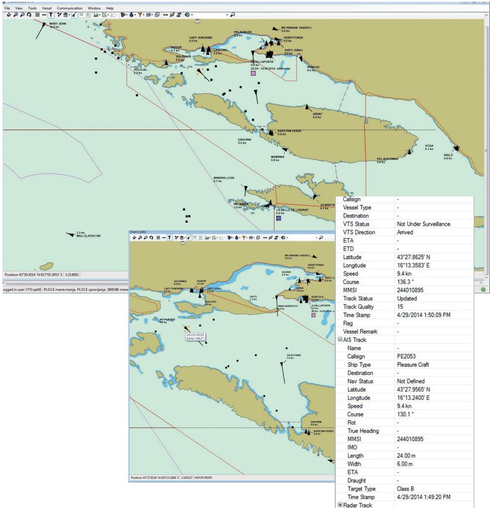
**Figure 7** Example of AIS B vessel/target display on Electronic Navigational Chart (ENC) (SAAB CoastWatch VTS Software)
