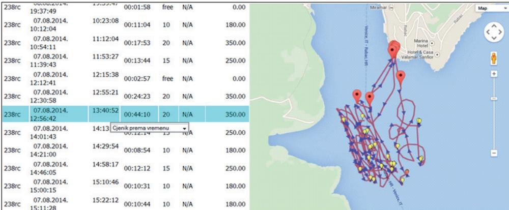
**Figure 8** Generated income report with one driver's session trajectory generated from logged data on one real location.
