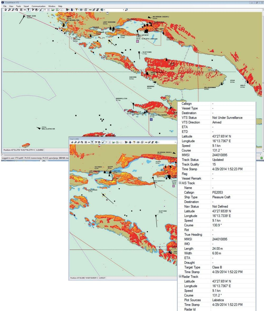
**Figure 8** An example of both radar and AIS monitoring of AIS Class B target displayed on Electronic Navigational Chart (ENC) (SAAB CoastWatch VTS Software)
