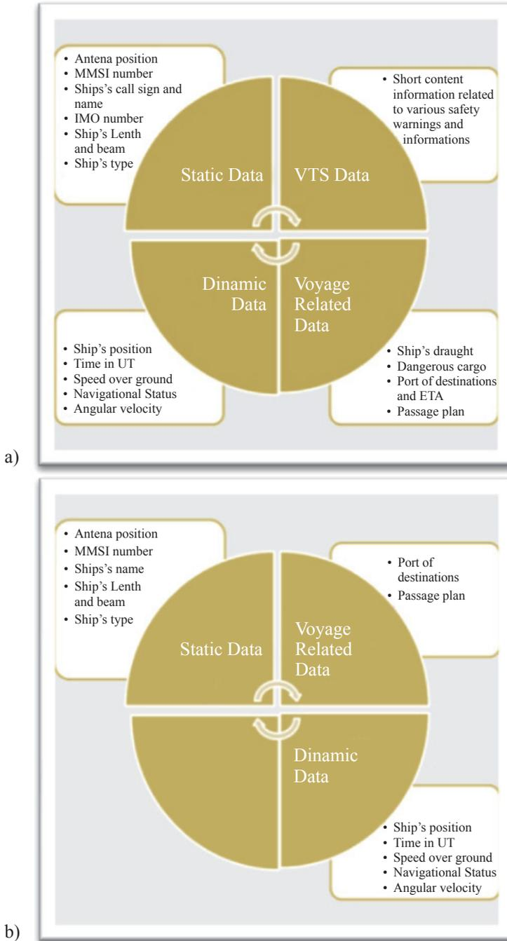
**Figure 2** Comparison of AIS Class A (a) and AIS Class B (b) information
