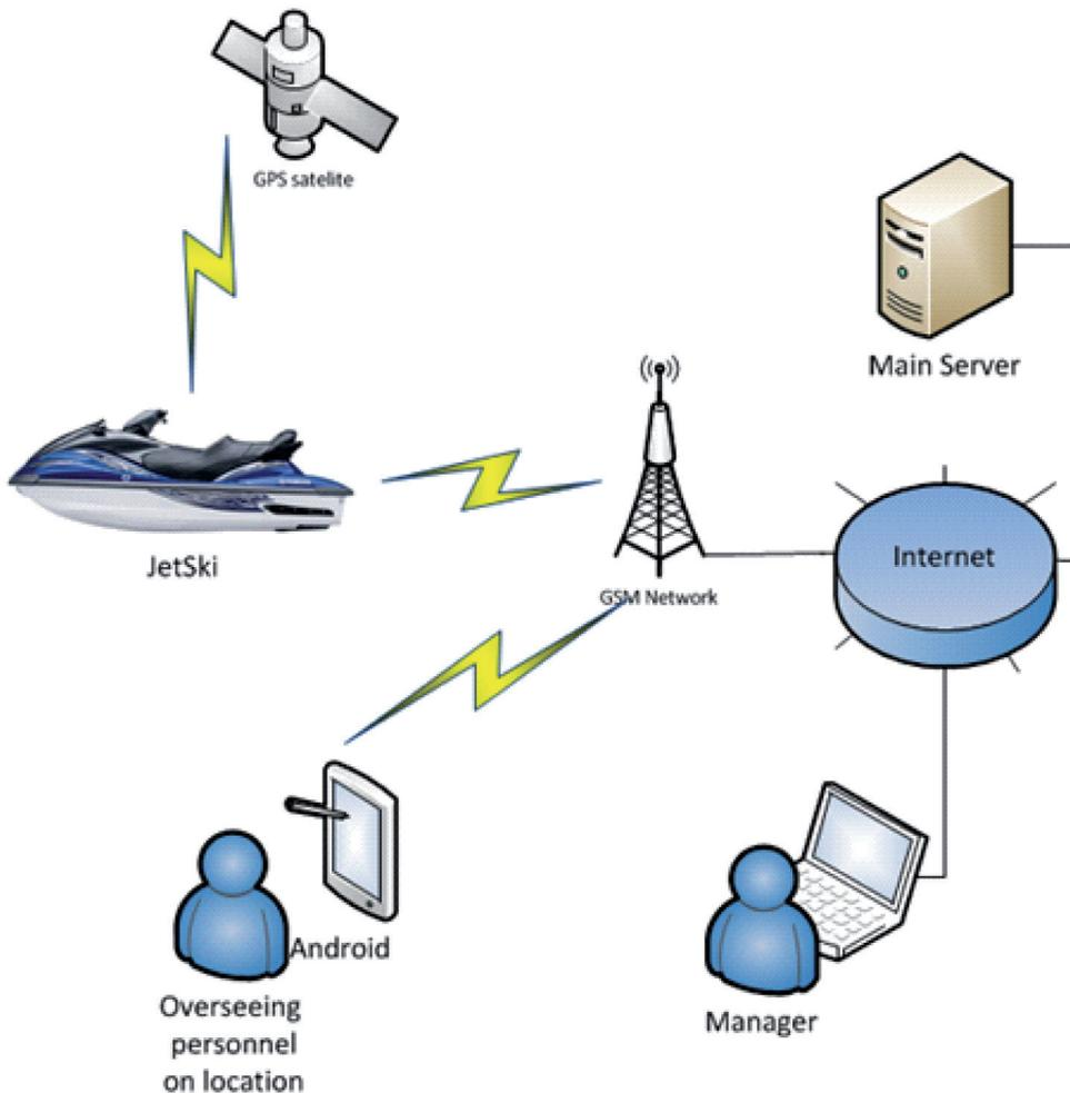
Figure 3 Block diagram of tracking system architecture
