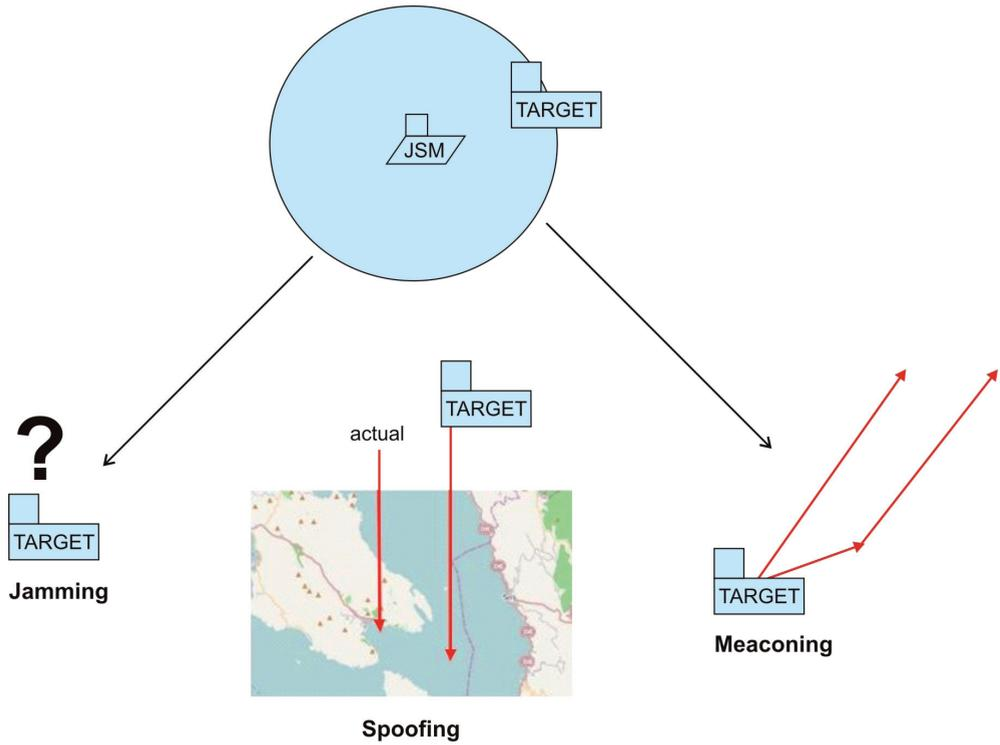
**Figure 1** Challenges of the open-sea satellite-based navigation
