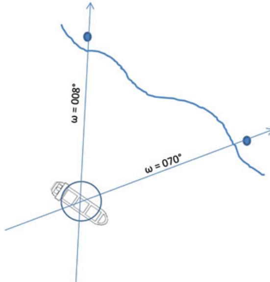
**Figure 1** Position fix with two bearings on conspicuous objects
