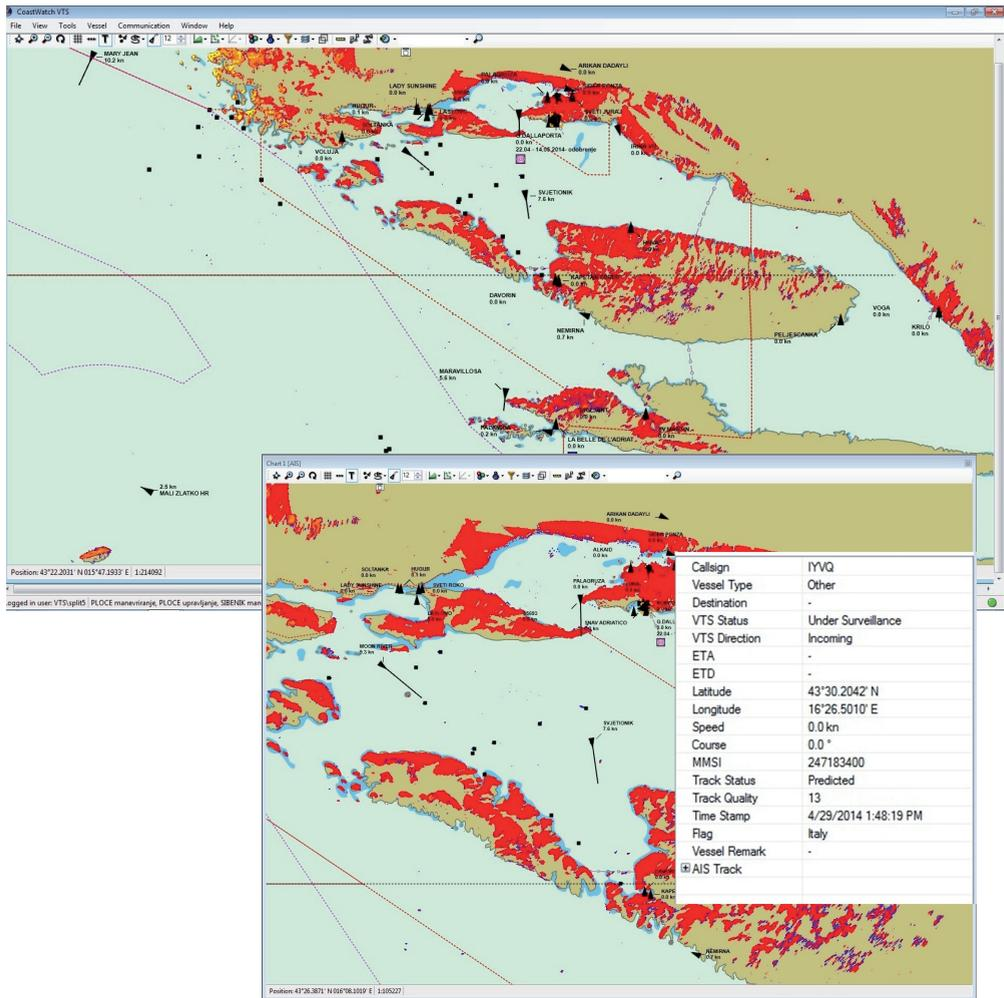
**Figure 6** Vessel Traffic Service AIS and radar tracking displayed on Electronic Navigational Chart (ENC). Example of research/survey vessel in port of Split (SAAB CoastWatch VTS Software).
