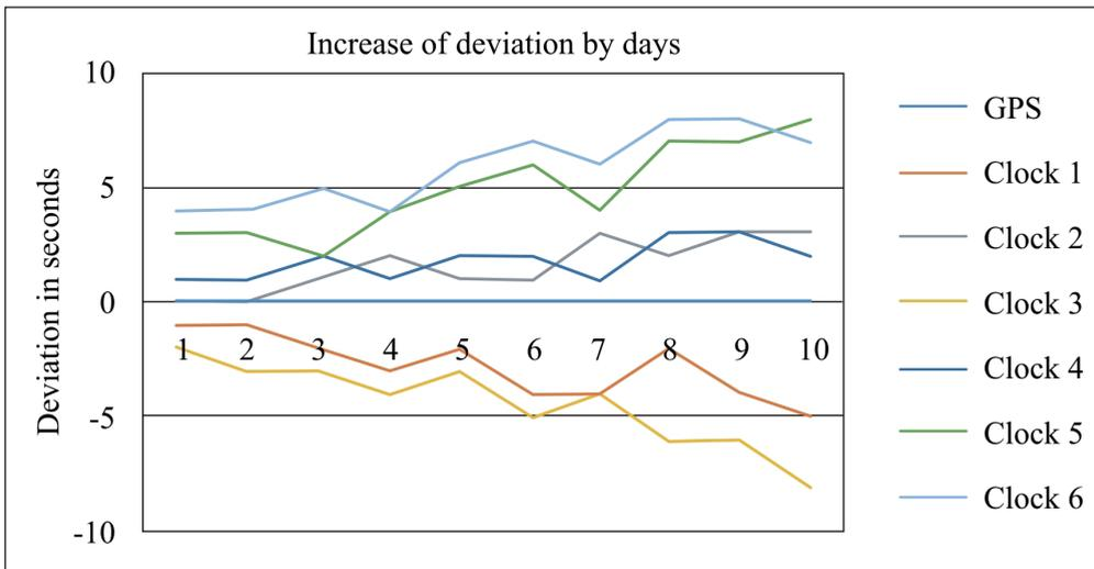
**Figure 4** Students' results of the 10 days testing of six clocks
