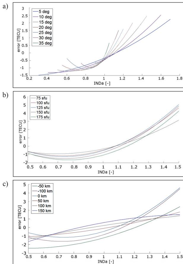
**Figure 8** Variation of mapping function error depending on asymmetry index for changing solar radio flux (a), elevation angle (b) and ionospheric height (c)
