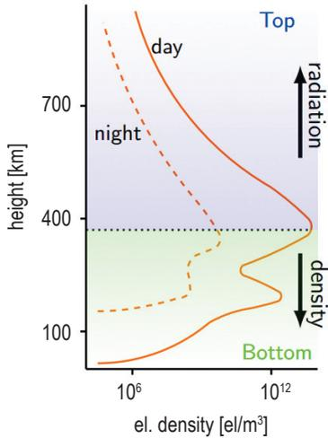
**Figure 1** A typical electron density vertical profile of the ionosphere. The electron density profile during day and night is represented by full and dashed line, respectively. The dotted line shows the average height of the electron density maximum; made by the authors according to Ya'acob et al., 2008.
