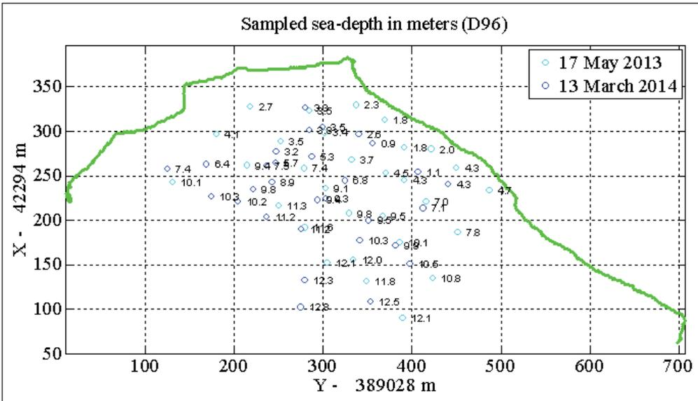
Figure 7 An overview of the sea-depth in meters near the faculty harbour in the local geodetic frame. Coastal line is coloured in green.
